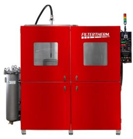
Specs: White Water Tank: 95 gal. capacity, Grey Water Tank: 40 gal. capacity. Electrical: 208VAC 3 phase, 30A GFCI protected breaker, I Equipment Dimensions: 96" W x 48" D x 96" H (includes filter tank & control panel) I Shop footprint: 120" W x 78" D x 96" H (with clearance for the doors), leave 12" to 18" from wall.
